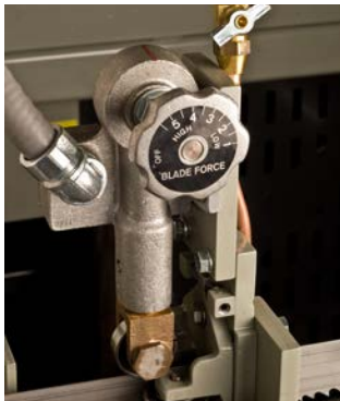
Automatic Cutting Force Control
