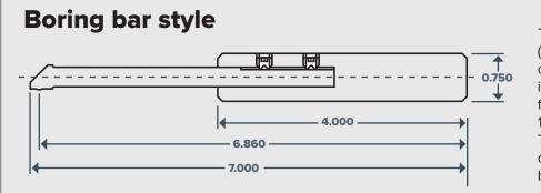
The boring-bar style tool (S2295-00) is designed for lathes or turning centers to provide an improved surface finish in bores from 0.500" to approximately 1.375" diameter x 2.800" deep. This burnishing tool can be used on most metals with a hardness below Rc40.
