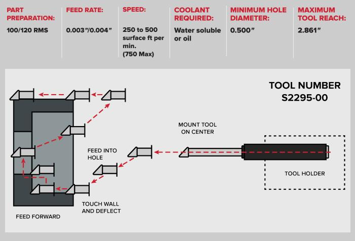
Can be used on most metals with a hardness below HRC40.
